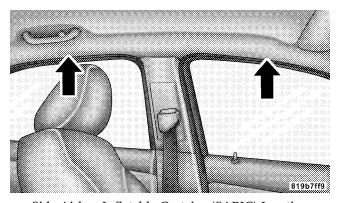
Side Airbag Inflatable Curtains (SABIC) Location
